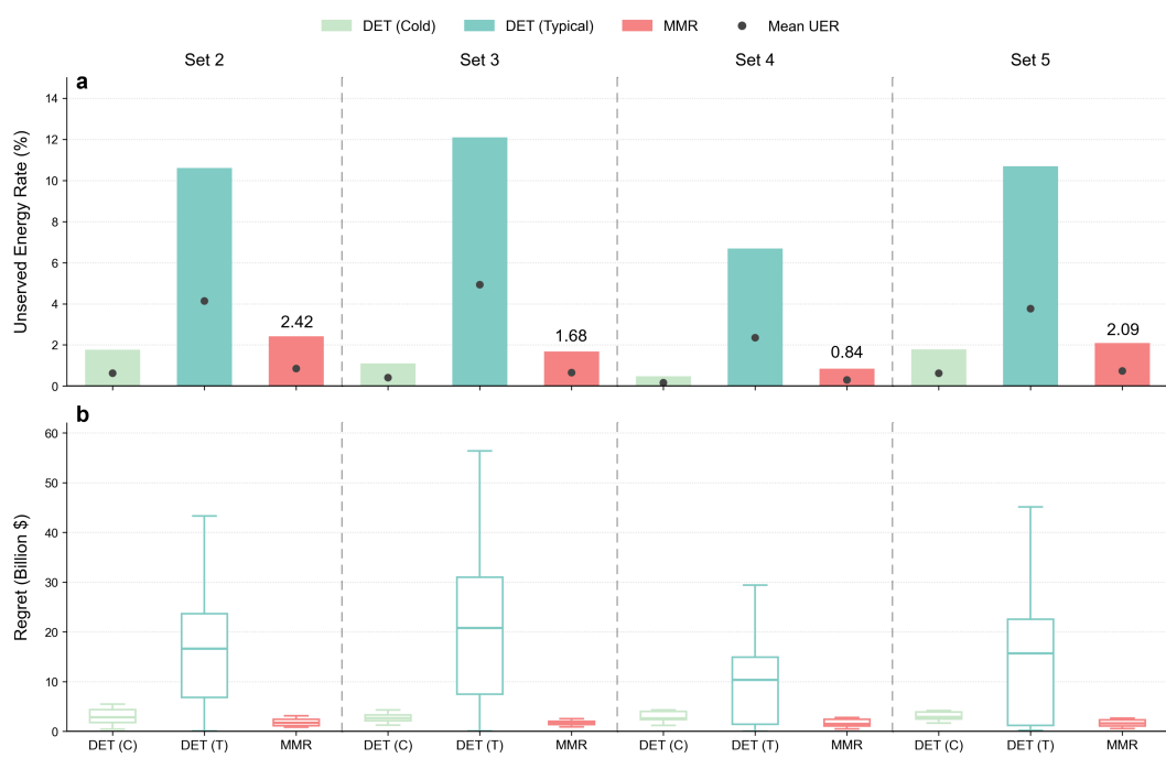
Figure 9: Cross-validation analysis of reliability and economic performance across independent validation sets. (a) Consistency of unserved energy rates showcasing maximum (bars) and mean (dots) values; (b) Distribution of economic regrets among deterministic and robust modeling approaches.
